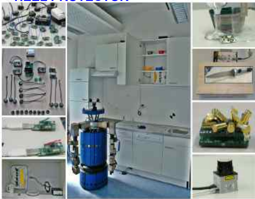
Fig. 1. The Assistive Kitchen containing a robot and a variety of sensors.
